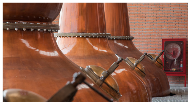
Copper stills used for the production of malt whisky
