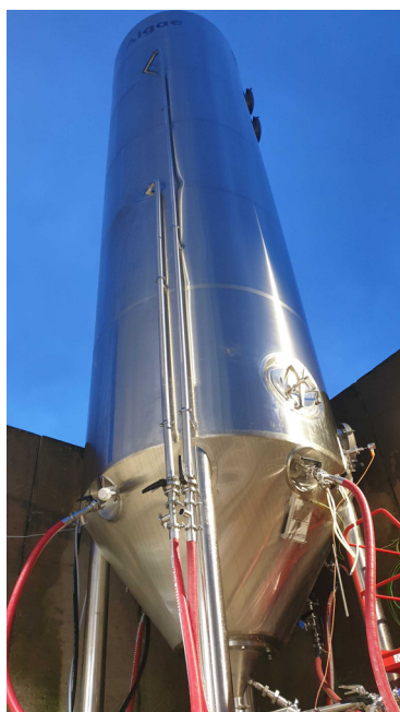
Special fermentation vessel for growing algae
